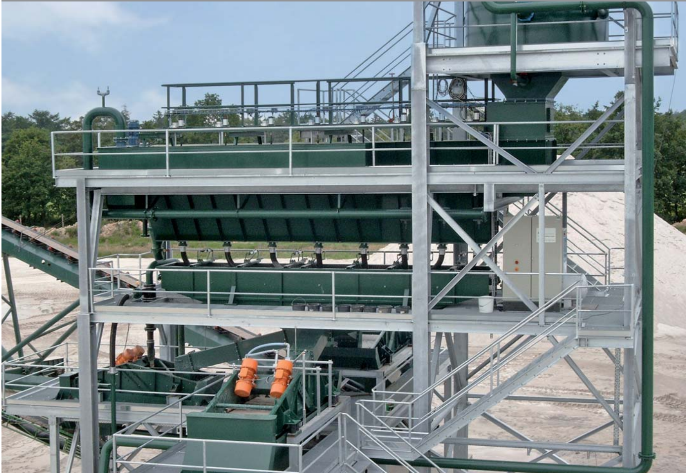
Freifallklassierer, Bauart AKOREL Free-fall Classifier, Construction AKOREL
